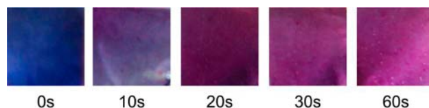
Figure 6. Time-dependent color changes of \text{PDA-1} -embedded electrospun microfibers in a \text{CO}_2 atmosphere saturated with TEA vapor.
